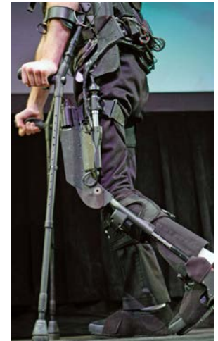
This lower-body exoskeleton, named eLEGS, is a bionic device that helps people with paraplegia stand and walk.
