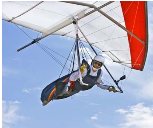
The glider's harness keeps the pilot's body straight to cut wind resistance.
