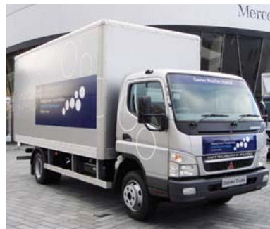
Mitsubishi Fuso Canter Eco Hybrid, diesel-electric
