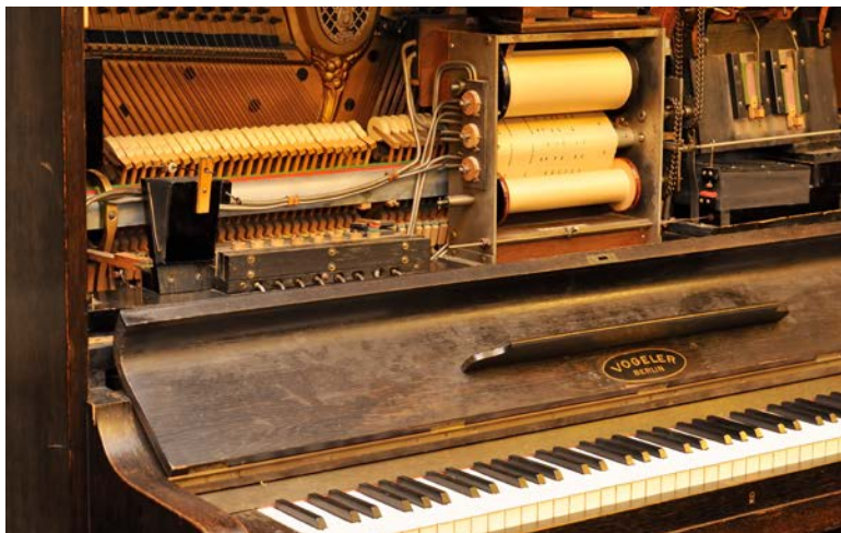
This player piano from the late 1800s is driven by an electric motor.
