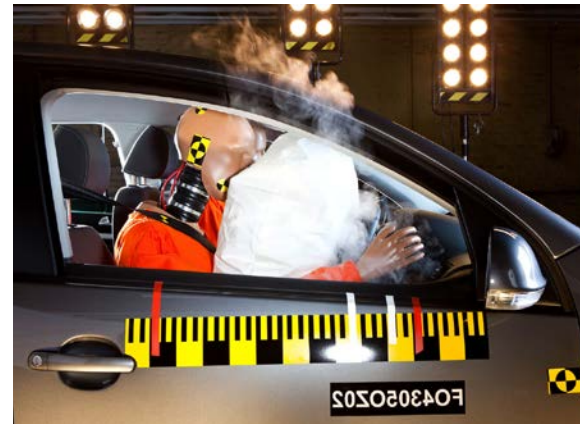
Carmakers see how well airbags work by using crash test dummies that look like humans.
