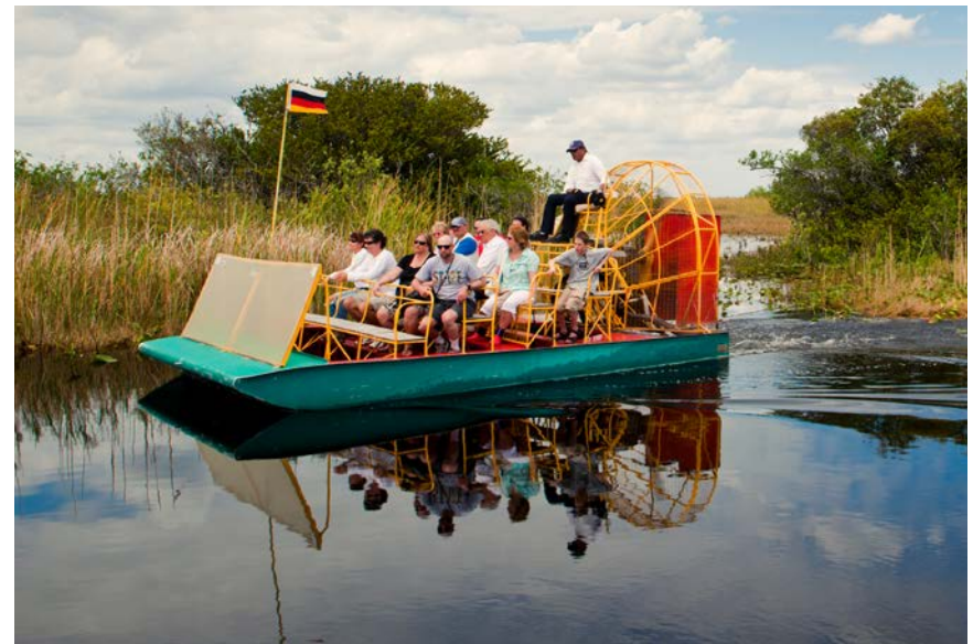
Airboats have flat bottoms that make travel across the shallow water in the Everglades easy.
